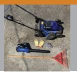
**Step 1:** When the swale is not excessively wet, mow grass to 3-6" high.
